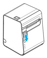
2. Insert the roll paper spacer so that the front edge goes through the notch; then push down the spacer so that the hook on the spacer and the shaft align.
