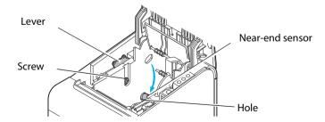
4. Tighten the screw and make sure the lever moves smoothly.
