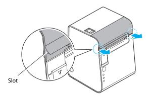
3. Turn the knob in the direction of the arrow in illustration, by using a ballpoint pen or tweezers, until you see a triangle mark in the opening.
