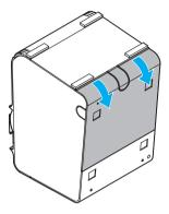
2. Break off by hand any of the three portions indicated by circles in illustration to pass the cables through.
